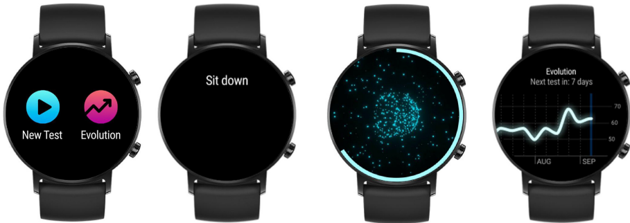
Fig. 2b. Core user interfaces of the smartwatch segment, where users are guided through a Sit-To-Stand protocol to measure their physiological stress levels.
