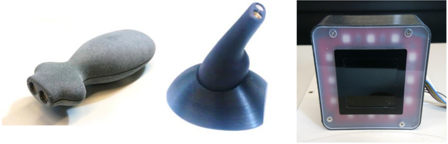
Fig. 2. (Left) Two version of the handheld, buttonless, battery-powered SmartPointer , based on user-centered design: a slim ‘cross’ (left) and a bulbous ‘pipe’ (right), with charging cradle. (Right) Receiver box with the array of IR sensitive photodiodes behind the optical filter (black square) to block ambient light, and a ring of in green and red LED for visual feedback. (Color figure online)
