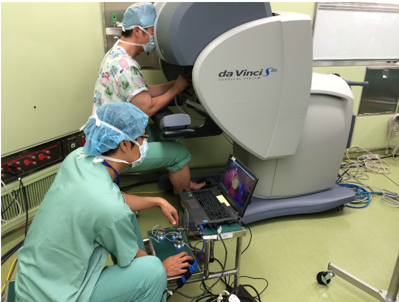
Fig. 1. Our previous system. The position and posture of the 3DCG were controlled with a mouse, and the transparency of each part of the 3DCG was controlled with three rotary controllers.
