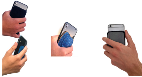
Fig. 9. The first three embodiments of working Holdable devices. From left to right: Holdable Original and Cover , Wave Up , Skinterface .
