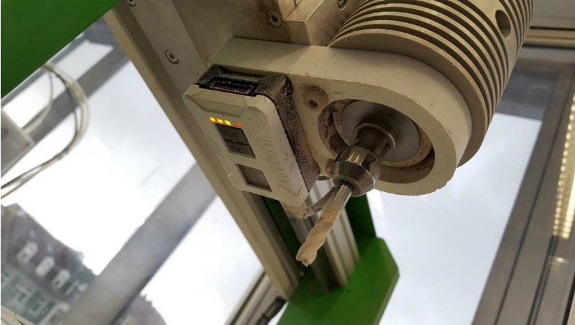
Fig. 1. Bosch XDK on the milling machine. Deposits on the sensor caused by the machining process can be seen here.
