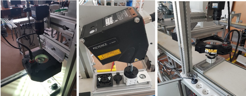
Fig. 6. 3D vision camera system with basic parts check (left), Multispectral vision system for surface error detection (middle), 3D profilometer for parts dimension check (right).
