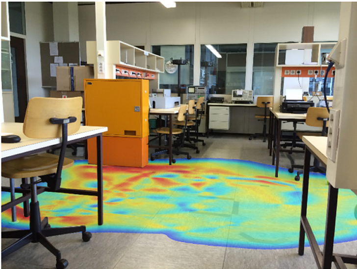
Fig. 9. Illustrative map of the horizontal flow of the laboratory for measuring and sensor technology
