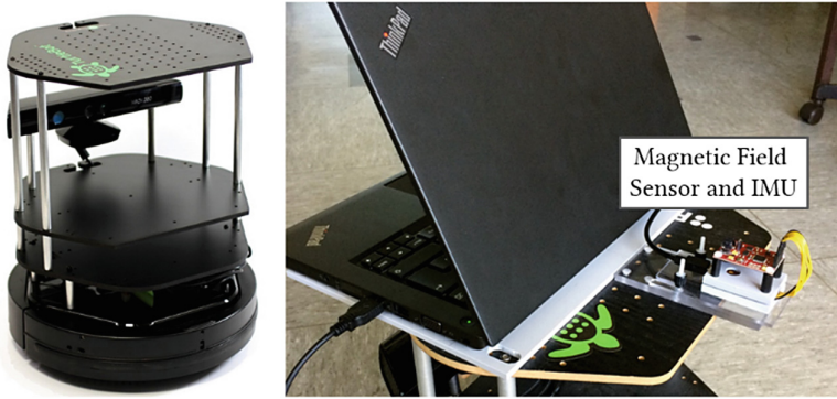
Fig. 4. Mobile robot platform (left) and experimental setup combined with magnetic field sensor IMU (right).
