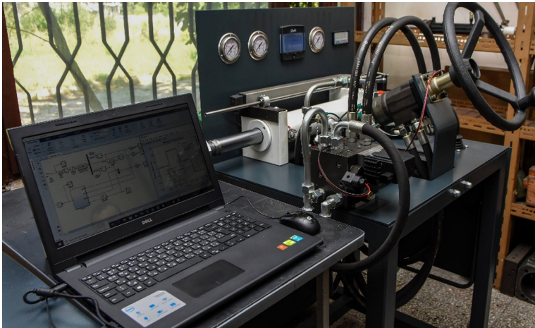
Fig. 1. Real implementation of laboratory electrohydraulic power steering test rig.
