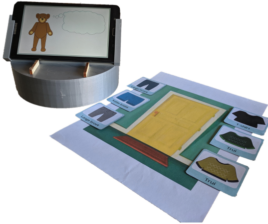
Fig. 2. Impression of the first prototype. The surfacebot with the character display is positioned next to one of the four locations with its associated clothes cards.
