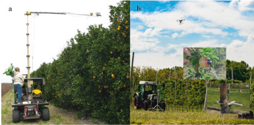
Fig. 8.3 Sensor platforms supporting optical sensors: (a) an agricultural vehicle and (b) unmanned aerial vehicle. Photographs courtesy of: Ehsani / Zude
