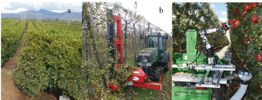
Fig. 8.2 Machine pruning in citrus (a) and apple (b) production, and harvester prototype (c). Photographs courtesy of: Zude / Betz / Karkee
