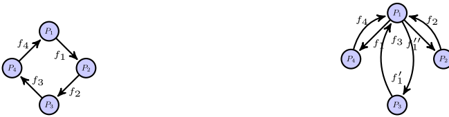
Fig. 1. Graph representation of the ring topology (left) and a random topology (right). f_i is the item of party P_i . The direction of the arrow shows the party who wants to receive it.
