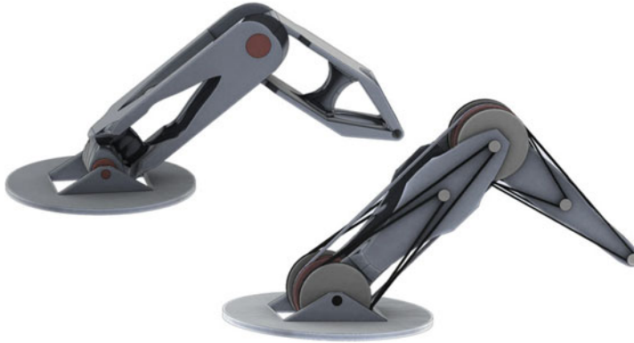
Fig. 6.9 Synthesized articulated arm robots derived by classical (left) and bioinspired approach (right) (Bartz et al. 2019)
