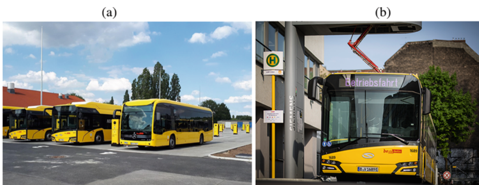
Fig. 7.9 (a) Depot charging (credit: BVG/Kevin Doan); (b) Opportunity charging (credit: Photothek)
