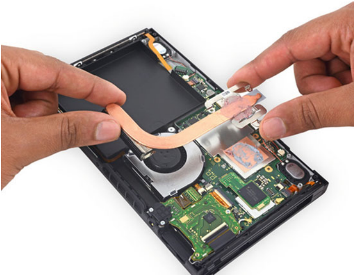
Fig. 4.9 Heat pipe connection on CPU from Nintendo Switch with thermal paste as a reference system (iFixit 2021)
