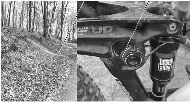
Fig. 1.2 Broken bushing support of the author’s mountain bike. The failure occurred during a downhill run in the Odenwald
