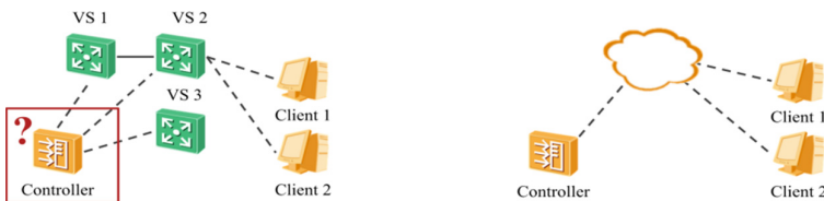
Fig. 5. Using smart access to organize a model network based on Open v Switch (controller and virtual switches).
