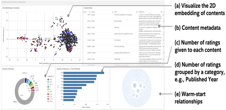
Fig. 4. Interactive visualization tool for item selection and exploratory analysis. Plot (a) visualizes the 2D embedding of items with trained items in blue, warm-started items in red and other untrained items in black; (b) shows the original content metadata such as Genre and Title; (c) and (d) show the feedback for each item or a group of items; (e) visualizes the warm-start relationships, such as how warm-started items are connected to trained items. (Color figure online)
