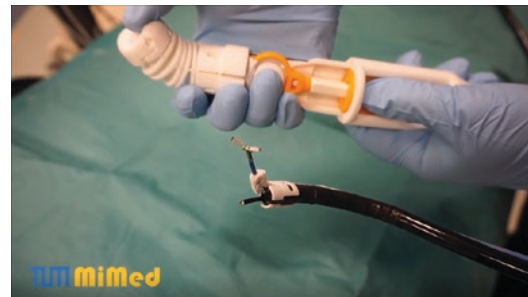
Fig. 26.2 Prototype of a hand-held device for tissue traction via an additional working channel
