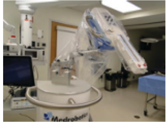
Fig. 29.3 The Flex® Cart is the other unit that makes up the Flex Robotic System that contains the Base and serves to give stability to the Flex® Drive, to transfer commands from the console to the flexible robotic arm. This system is compatible with both Flex® Drive flexible robotic endoscopes for transanal and transoral surgery
