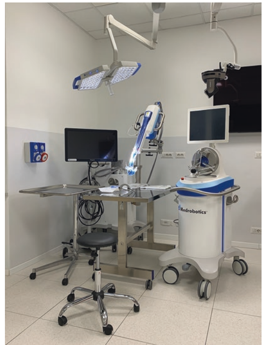
Fig. 29.1 Flex® Robotic System consisting of two transportable main units and a flexible robotic endoscope
