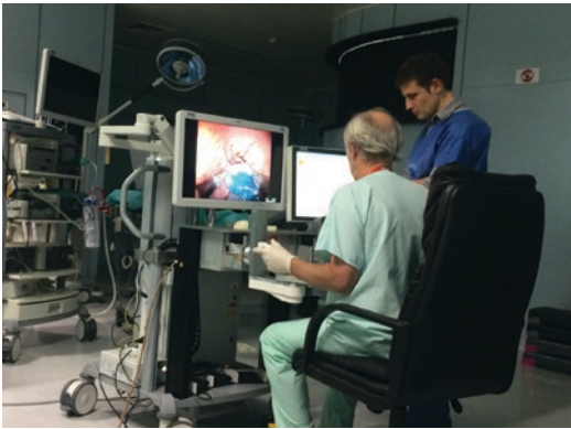
Fig. 6.5 Master unit of the Endoluminal Assistant for Surgical Endoscopy tele-operation by Dr. Bernard Dallemagne during a colonic ESD in a preclinical trial; notice the open joysticks which allow for arms control
