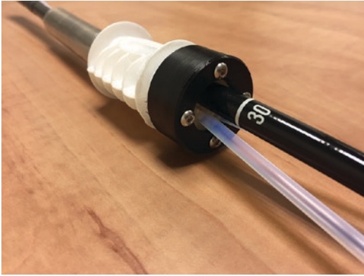
Fig. 23.3 Overtube adaptor design to facilitate insertion of endoscope and instruments through individual channels, while maintaining insufflation
