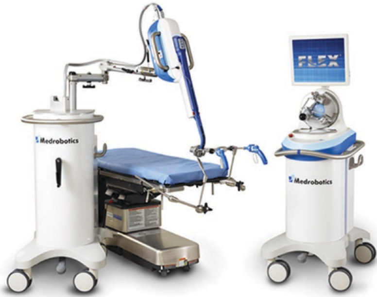
Fig. 1.14 The Flex robotic system with patient cart and single-port control [78]
