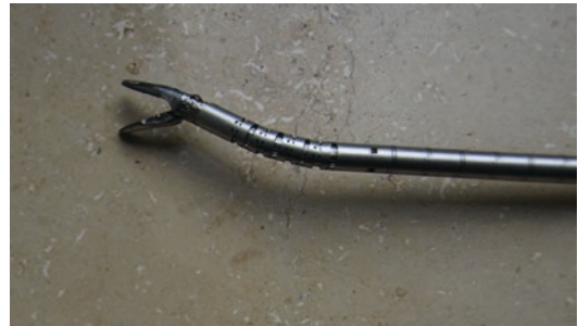
Fig. 13.2 End effector of the prototype needle holder for endoscopic procedures
