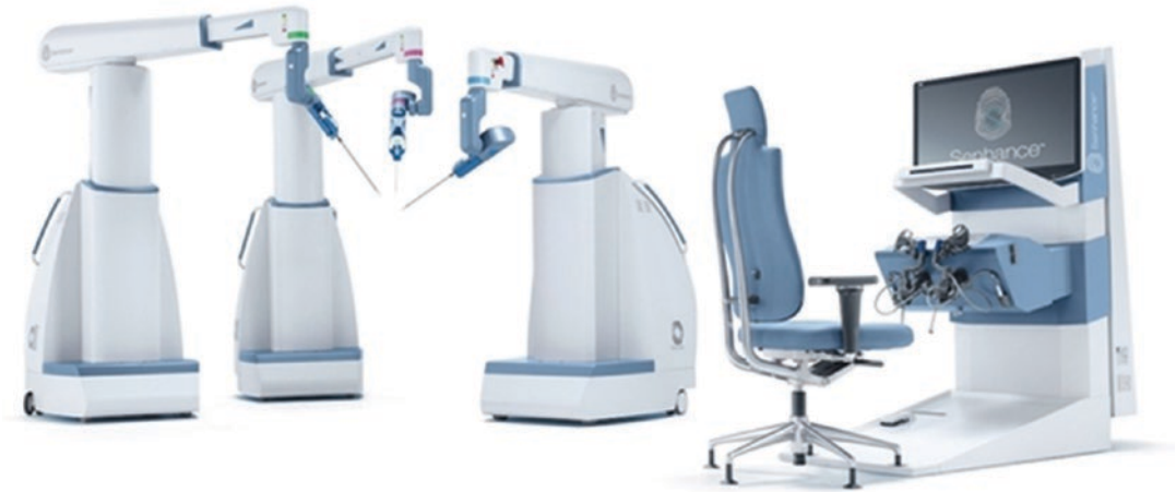
Fig. 1.6 Senhance® (TransEnterix, Morrisville, NC) surgical system with digital laparoscopy [33]
