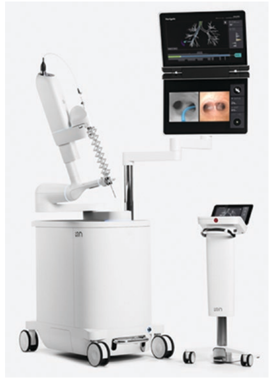
Fig. 1.5 The da Vinci Ion system for robotic lung biopsy [27]
