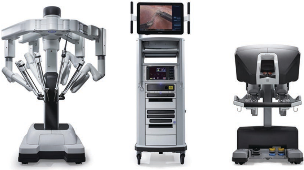
Fig. 1.3 The three basic components of the da Vinci telerobotic system – the surgeon’s console, video cart, and four-armed patient cart [20]
