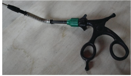
Fig. 13.1 Handle of the Fortimedix Surgical™ needle holder following the laparoscopic paradigm. It is used to grasp the needle and also by angulation and turning to steer the end effector
