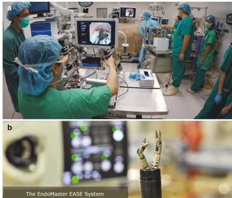
Fig. 6.7 (a) Setting of EndoMaster EASE system (Endomaster Pte Ltd., Singapore). (b) Endoscope and effectors for distal arms. With permission from Endomaster Pte Ltd. ( http://www.endomastermedical.com )
