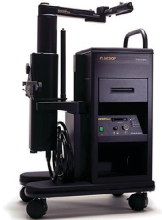
Fig. 1.2 AESOP®, a voice-controlled robotic endoscopic positioning system, provides an absolutely steady picture during minimally invasive surgeries [11]
