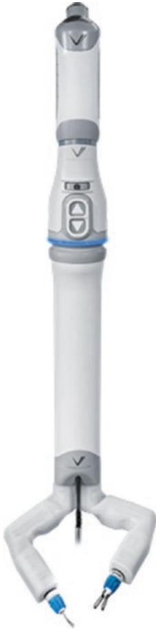
Fig. 1.9 Virtual Incision Corporation’s MIRA (“miniaturized in vivo robotic assistant”) [54]
