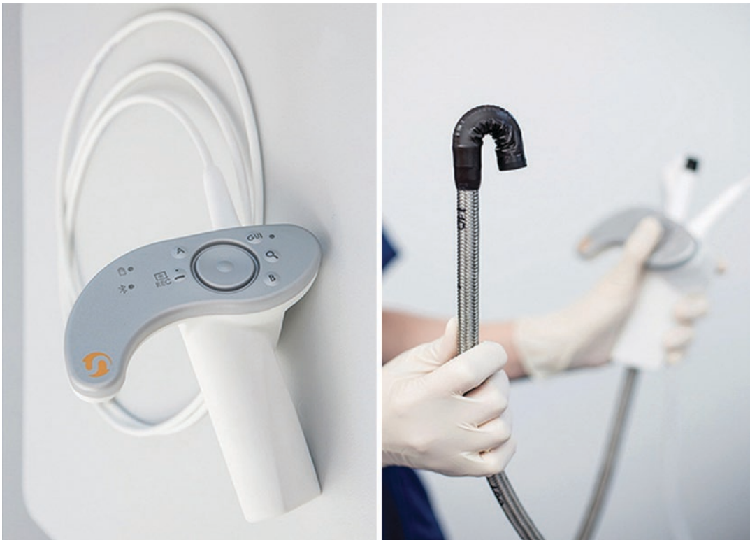
Fig. 1.13 The Invendoscope handheld propulsion unit with single-use insertion endoscope [74]
