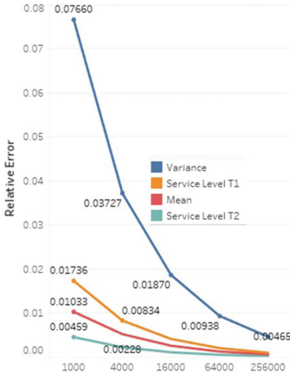
Fig. 6.5 Relative errors in simulations of Model 1 for different risk measures and values of m
