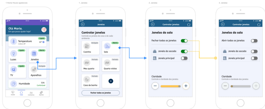
Fig. 6. User flow of Task 6. Control windows. As it is a cold day outside, you want to close the living room windows without getting up there.
