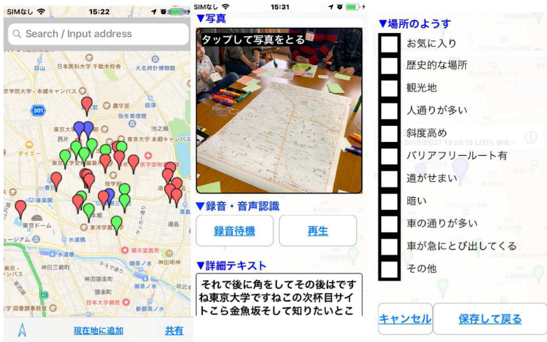
Fig. 3. The user interface of the mobile data recording application for assessments. The left figure shows the map view, and the middle and right figures show the data input views.
