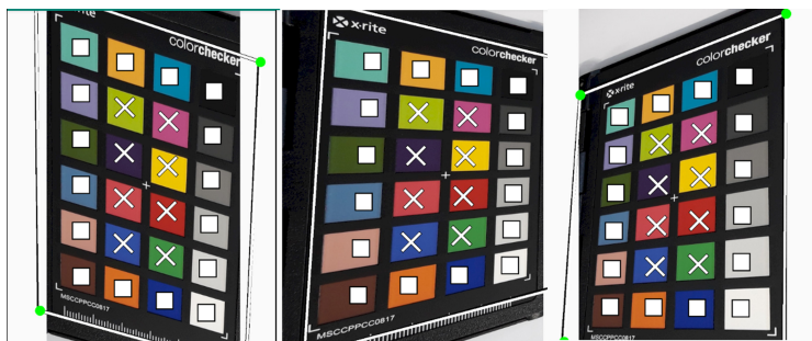
Fig. 7. Warping with manual patches detection.
