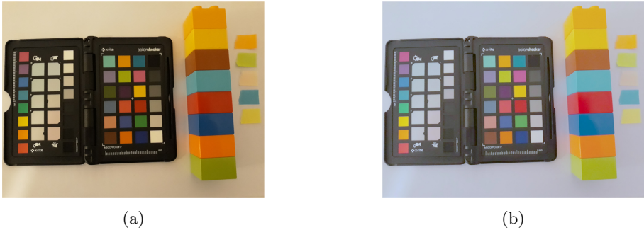
Fig. 1. Example of color correction algorithm using root-Polynomial regression. a) original photo, b) photo after correction
