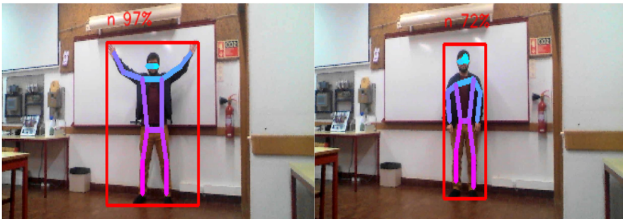
Fig. 2. Example of using the GluonCV estimator with its 17 joints, connected by lines, and the respective average accuracy.
