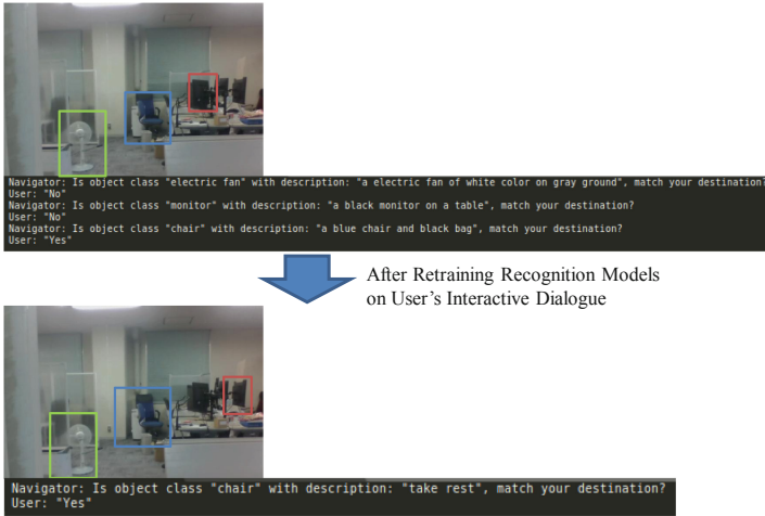
Fig. 2. A navigation task with the user’s spoken destination, “Where can I take rest”. In the initial time of navigation, the user’s destination was known after three times of dialogues (the above case). After personalizing by re-training recognition using interactive dialogues, in the next time of navigation, the user’s destination could be quickly known (the below case).
