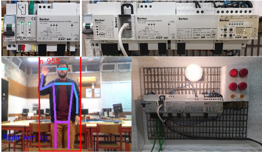
Fig. 4. Top row, detailed image of the KNX IP router (left) and devices (right). Bottom row, detection of a swipe-up (left), and the activation of the KNX device – lamp (right).
