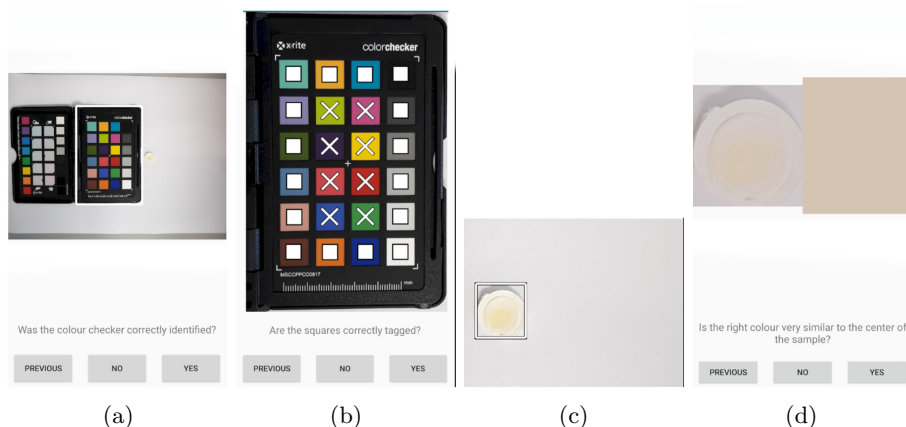
Fig. 5. Snapshots after running the algorithm automatically. a) color checker segmentation, b) patches segmentation, c) disk segmentation, d) sample segmentation.
