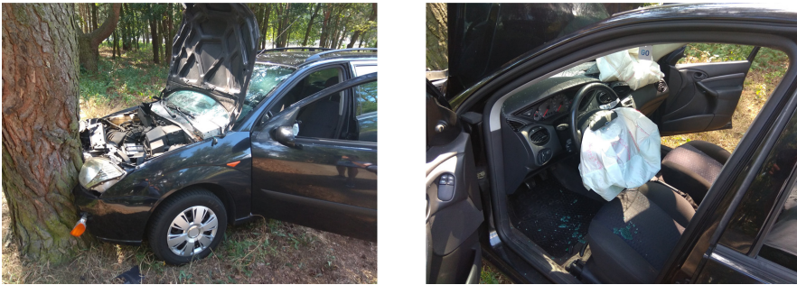
Fig. 2. Results of the collision with a tree (27.7 kph).
