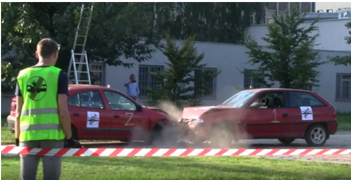
Fig. 1. Head-on collision at 40.3 kph.
