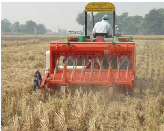
Fig. 11.2 The 9-row Turbo Happy Seeder sowing wheat into rice residues in a farmer's field. (Photo courtesy: BISA-CIMMYT, India, Sidhu et al. 2015)
