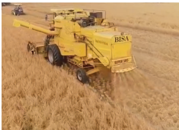
Fig. 11.3 Rice loose straw management by super straw management system attached to combine harvester. (Photo courtesy: BISA-CIMMYT, India)
