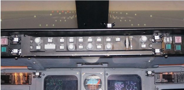
Fig. 2. Mode Control Panel (MCP) is the link between the pilots and the Autopilot flight Director System (AFDS)
