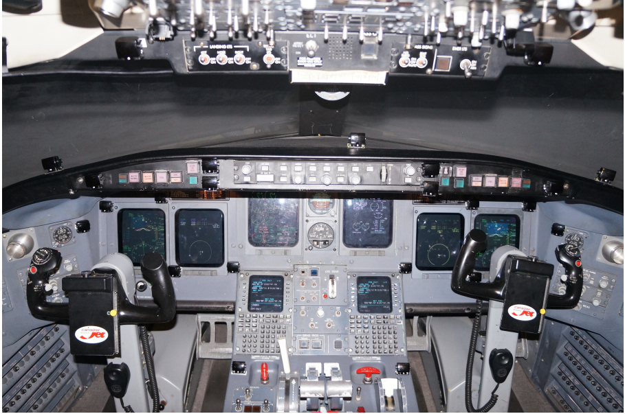
Fig. 1. The flight simulator used in our experiment. It is completely built according to the cockpit of the CRJ-200 aircraft
