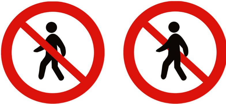
Fig. 2. Example of a pair of prohibitions signs with different bar positions: “No Entry” signs with bar as foreground (left) and bar as background (right).
