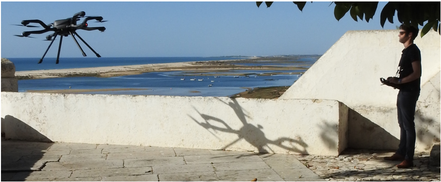
Fig. 1. A TNO reconnaissance drone departing for BVLOS flight during the (now concluded) EU funded ALFA (Advanced Low Flying Aircrafts Detection and Tracking) project [5] where it facilitates automatic threat evaluation for border security and surveillance. The pilot uses the control interface to see what the drone can see.
