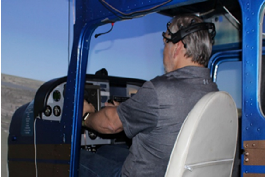
Fig. 1. Environment and interior of full-scale Cessna 172 flight simulator (left door removed).
