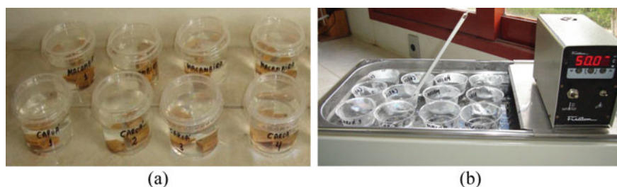
Fig. 3.6 a Caroá and macambira composite specimens and b Macambira and caroá composite samples in water bath
