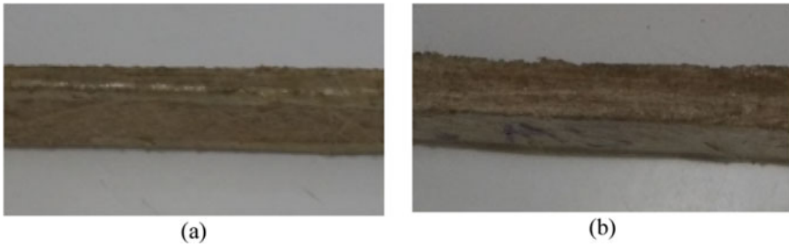
Fig. 3.21 Sisal fiber-reinforced polyester composite (44.6% sisal fiber) at saturation condition ( T = 25\text{ }^{\circ}\text{C} ). a 3 mm and b 6 mm thickness
