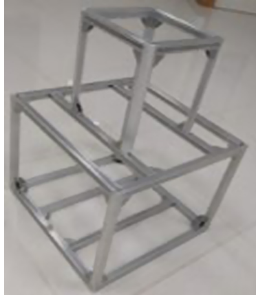
Fig. 4. Chassis with aluminum profiles
