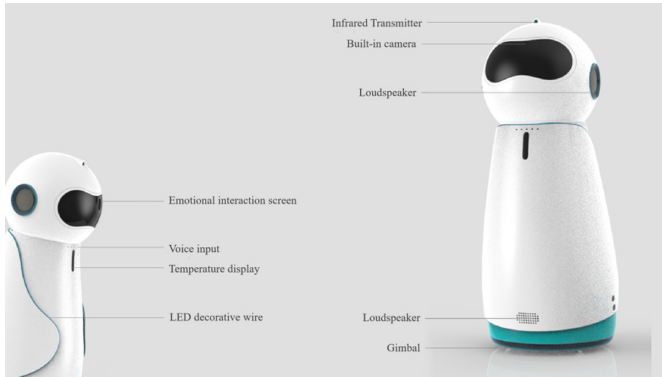
Fig. 11. Guided robot's structure
