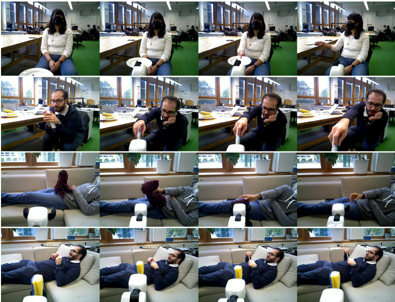
Fig. 3. Trials the handover functionalities consist of successful handovers, failed trials including unreleased objects, dropped objects, and ignoring the robot (top to bottom)
