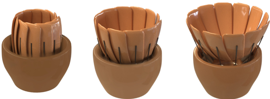
Fig. 4. Simulation of the opening of the prosthetic socket
