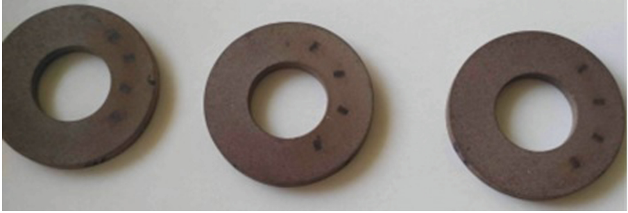
Fig. 2. Samples synthesized on the 2024 alloy after a friction test.
