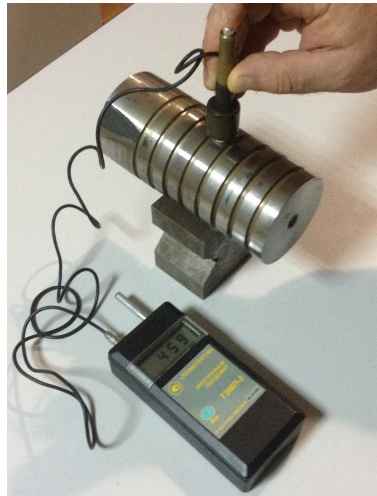
Fig. 7. Experimental study of the machined surface layer microhardness of the alloyed steel workpiece (X40CrMoV5).
