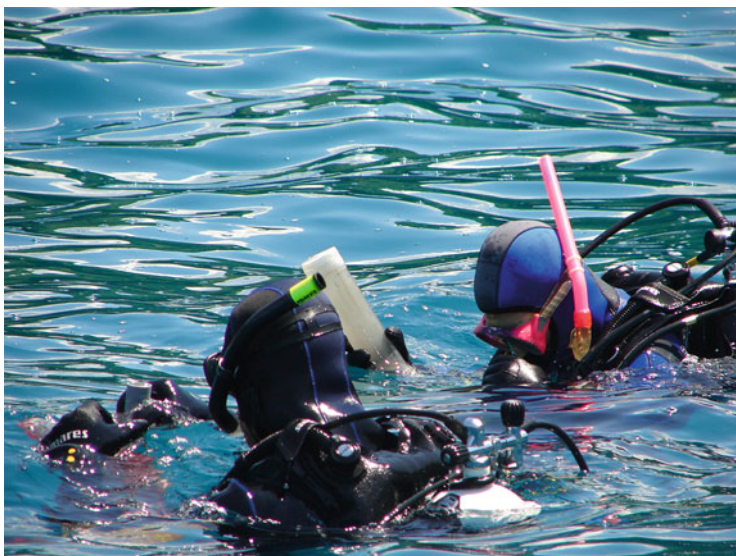
Fig. 4 Sediment sampling by autonomic divers with plastic tubes of corer (Photo by S. Matijević)
