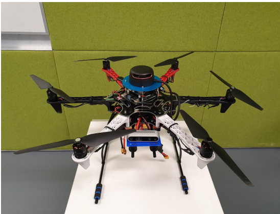
Fig. 2. Our drone configuration with integration of RPLidar A2 (bottom left) and Intel RealSense D435i (bottom right).
