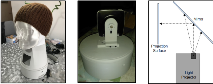
Fig. 1. Robot head design solutions: (1) PLEA - physical robot design, (2) light pico projector fixed at the robot base, and (3) light projection solution.
