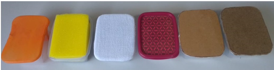
Fig. 1. Real materials used in the experiment (from left to right): rubber, sponge, fabric, plastic, cardboard and wood.
