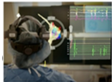
Fig. 6. SentEGM System. In this prototype of the SentEGM system, the user wears a Microsoft HoloLens HMD and is able to see the electrogram data alongside the CommandEP map data.
