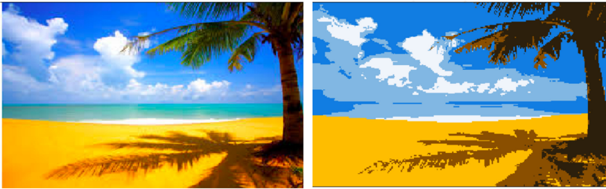
Fig. 2. Input image for processing and the result of segmentation by the k-means method.
