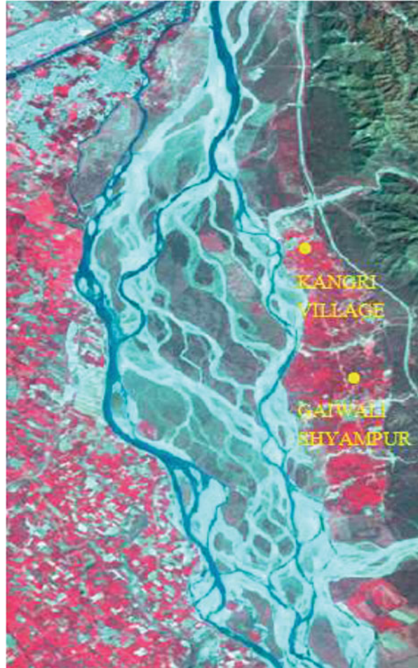
Fig. 8.8 LISS IV image of Ganga River indicates extensive braided channel in downstream (near Laksar) and in upstream (near Haridwar) comparatively confined channel observed due to structural control. (Source: LISS-IV, 2005, NRSC)
