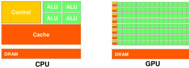
Fig. 3. Diagram of CPU and GPU structure.
