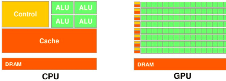
Fig. 3. Diagram of CPU and GPU structure.
