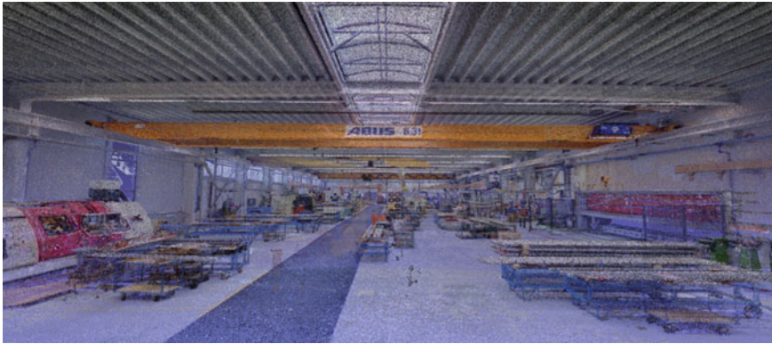
Fig. 8.8 Factory hall as a point cloud scene
