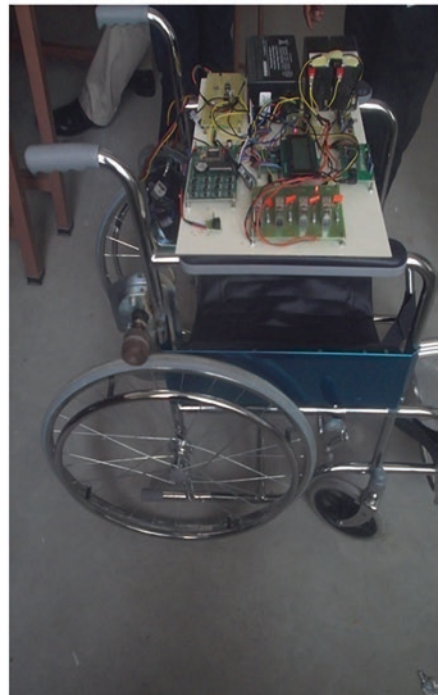
Fig. 13 Wheelchair with heartbeat measurement, temperature measurement, and respiratory rate kit
