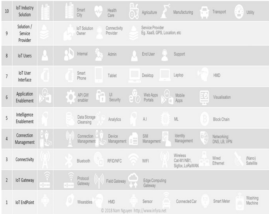
Fig. 1 10-layered IoT architecture with “IoT Industry and Solution” at the top and layer 1 “IoT Endpoint” at the bottom
