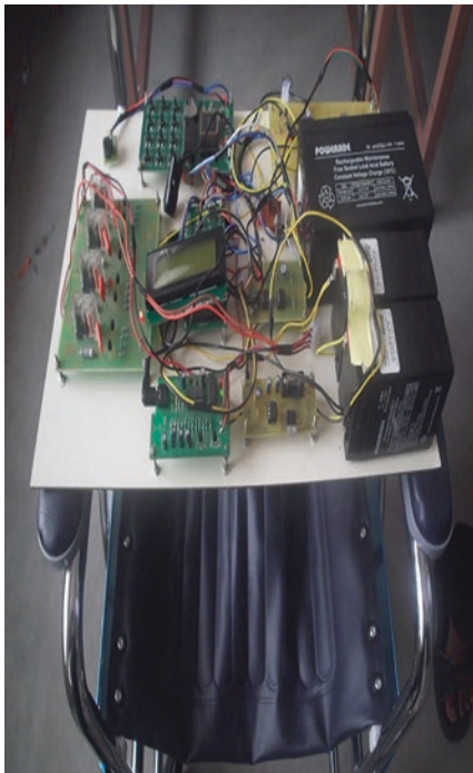
Fig. 13 Wheelchair with heartbeat measurement, temperature measurement, and respiratory rate kit
