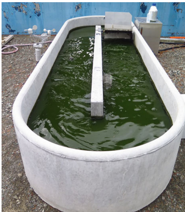
Fig. 5 Concrete 1,000 L HRAP located in Palmerston North, New Zealand. Courtesy of Dr. Andrea Hom-Diaz
