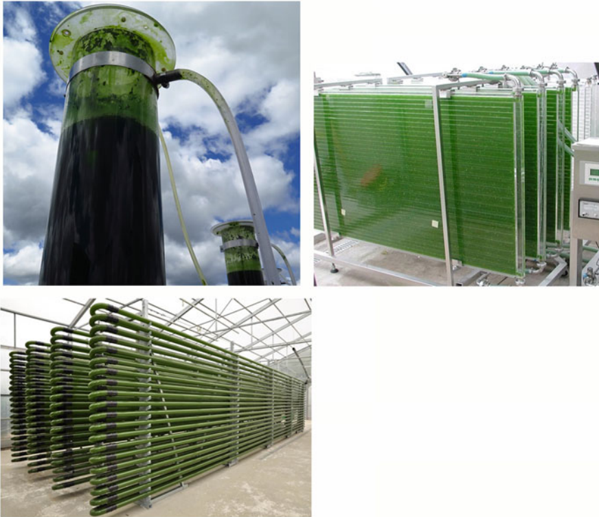
Fig. 2 Microalgal closed photoreactors. Top: vertical column; Bottom left: flat panel; Bottom right: horizontal tubular
