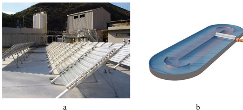
Fig. 2 View of CPCs (a) and basic schematic concept of RPR (b)
