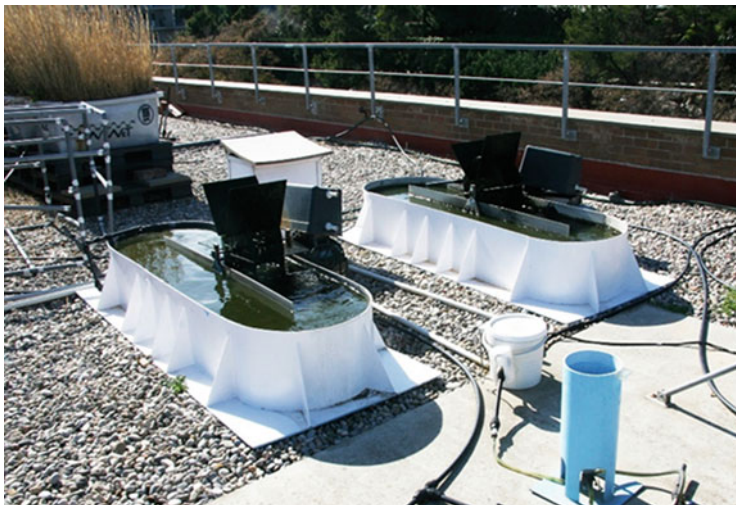
Fig. 7 470 L HRAPs located outdoors at the laboratory of the GEMMA research group (Universitat Politècnica de Catalunya – BarcelonaTech, Spain). Courtesy of Dr. Ivet Ferrer
