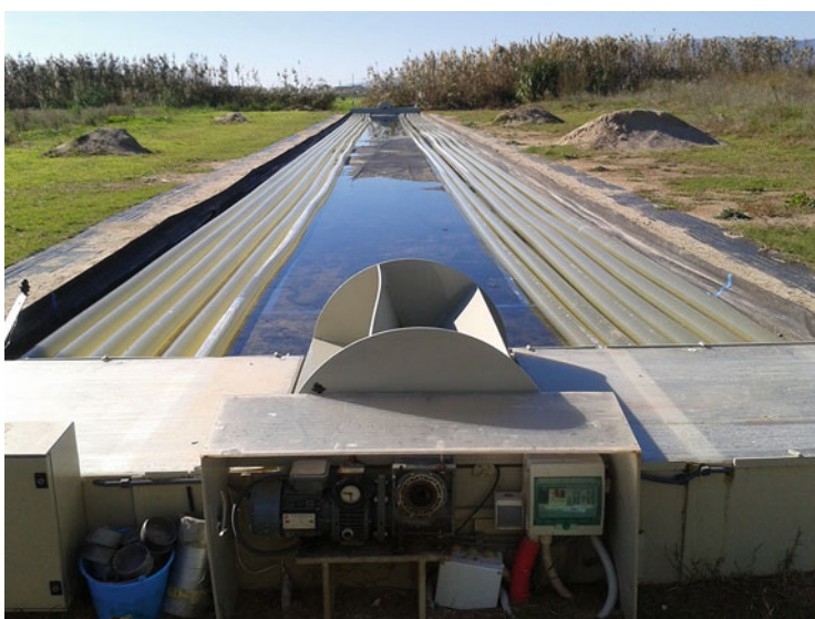
Fig. 8 Full-scale semi-closed tubular PBR located in Agropolis, Barcelona, Spain. Courtesy of Dr. Ivet Ferrer
