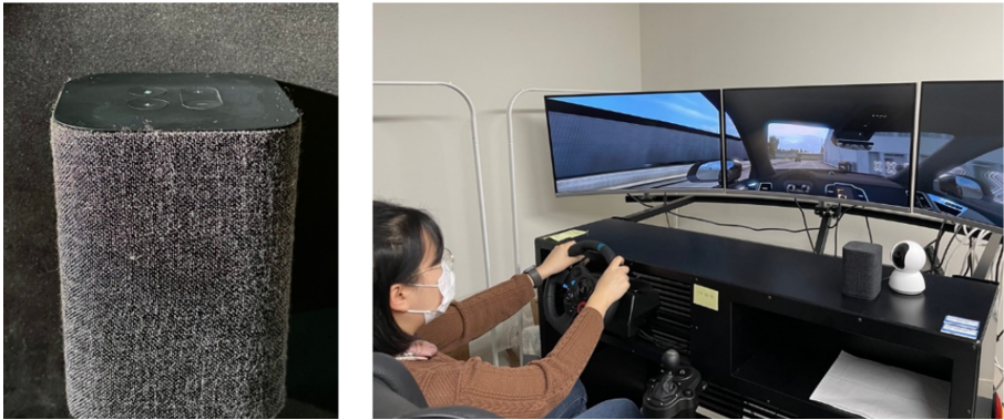
Fig. 2. Driving simulator environment (left: bluetooth speaker used in the experiment/right: experiment participant running in a simulator)
