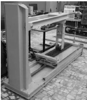
Fig. 3 The test stand involved in the experimental tests on motion resistance of double-flanged rollers carried out in the laboratory of DORMVE at Wrocław University of Science and Technology
