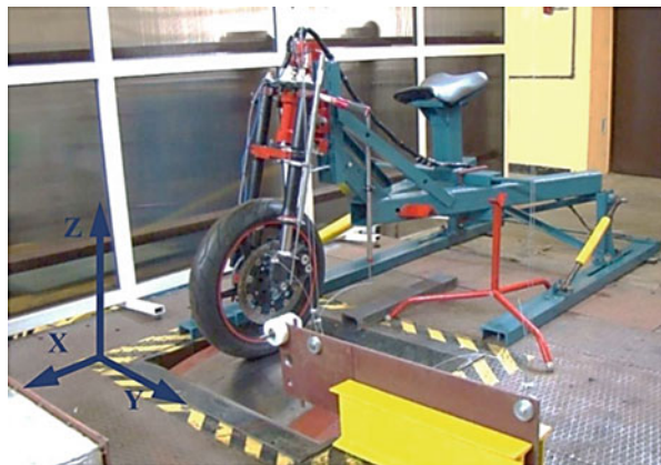
Fig. 1 Test stand of motorcycle steering system
