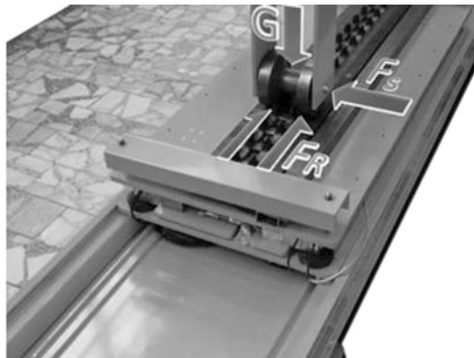
Fig. 3 The test stand involved in the experimental tests on motion resistance of double-flanged rollers carried out in the laboratory of DORMVE at Wrocław University of Science and Technology
