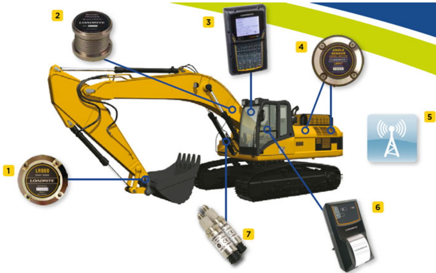
Fig. 1 Components of the Load Rite X2350 payload monitoring system by Trimble [3]: 1, 2 – inclination sensors for determining the angular position of the bucket and boom, 3 – control panel, 4 – ground inclination sensors, 5 – wireless data transmission device (wi-fi, GPRS, radio communication), 6 – printer, 7 – oil pressure sensors
