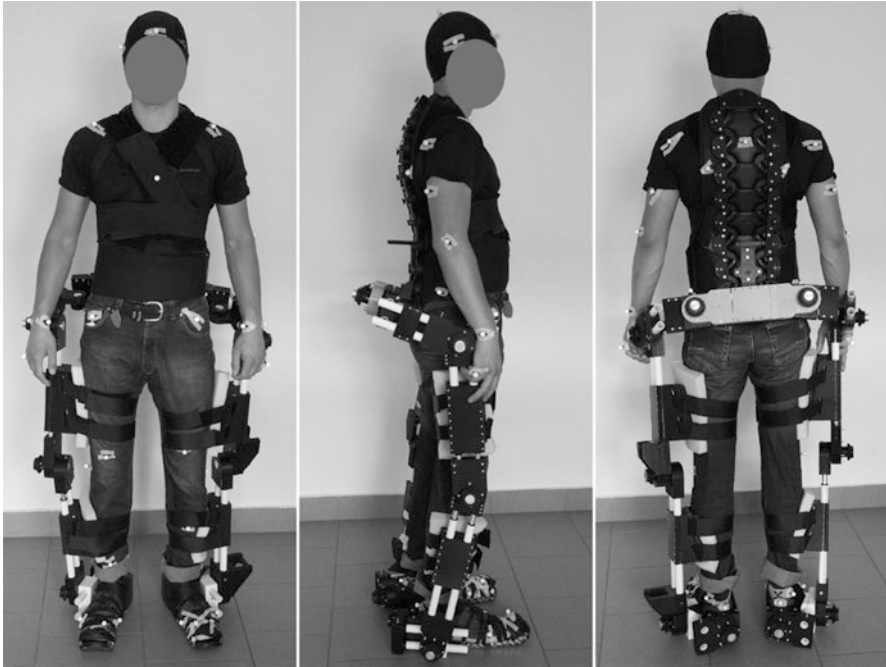
Fig. 6 Passive prototype of the developed exoskeleton. Front view (on the left), side view (centre), rear view (right)
