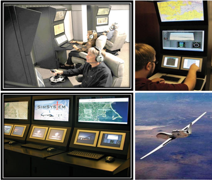
Fig. 4.2 The RPAS research testbed: RPAS-STE: remotely piloted aircraft system (ground control station) synthetic task environment. In our RPAS-STE, three human operators must interdependently coordinate their actions over headsets or text chat messages to be able to maneuver their RPA under their control to take pictures of selected ground targets based on intelligence or other requests. Clockwise from the lower right-hand image is shown a remotely piloted drone (pictured: A Northrop Grumman RQ-4 Global Hawk; it is a high-altitude, remotely-piloted, surveillance aircraft ). At the bottom-left is an image of experimenter control stations for the RPAS-STE. At the upper-left is an image of three human operators interdependently in action. And at the upper-right is an image of an operator controlling a RPA drone
