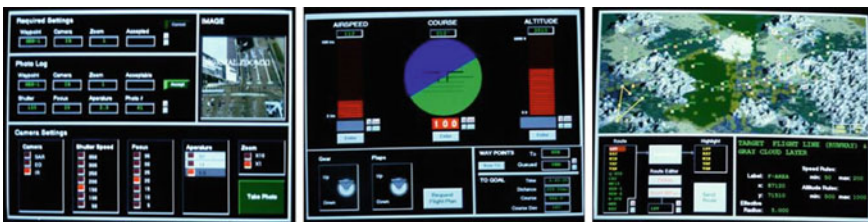
Fig. 4.3 A Remotely Piloted Aircraft System (RPAS) ground control station can be located almost anywhere, but principally on the ground or on a ship. Here screenshots from the Cognitive Engineering Research on Team Tasks (CERTT) RPAS Synthetic Task Environment (STE) are provided: (Left) The left-hand screen image is an image from a screenshot of a Payload Operator’s station and what is commonly seen in a real-time video in its upper-right portion; the Payload Operator controls the various camera settings, takes photos of selected objects or targets, and monitors the different camera systems. (Center) A screenshot of an image from the Data Exploiter Mission Planner’s work station is shown; the DEMPC is the navigator, mission planner, and route planner from target to target. (Right) A screenshot taken of an image from the Air Vehicle Operator work station where the controls for the RPA’s airspeed, heading, altitude, and air vehicle systems are maintained and monitored
