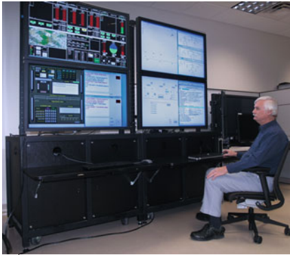
Fig. 4.4 A Synthetic Teammate Demonstration System (installed at Wright Patterson Air Force Base, Dayton, OH; see Ball, Myers, Heiberg, Cooke, Matessa & Freiman, 2009). Results: The largest cognitive model built-in ACT-R. In ACT-R, it had 2459 Productions and 57,949 Declarative Memory chunks. Among the largest cognitive models built in any cognitive architecture at the time, it had five major components. By computer science standards, it was a very large program. (Left image) Facing the human operator, at the upper left, a computer screen-shot of the images seen is those of the CERTT Consoles (i.e., the Navigator; Photographer; Pilot). At the bottom left facing the human operator is shown the text messaging subsystem. At the upper right top and bottom, screenshots are shown of the Synthetic Teammate. (Right image) To the right is a series of actual texts captured between the human operators and the Synthetic Teammate (highlighted in yellow) as it communicated with its human teammates
