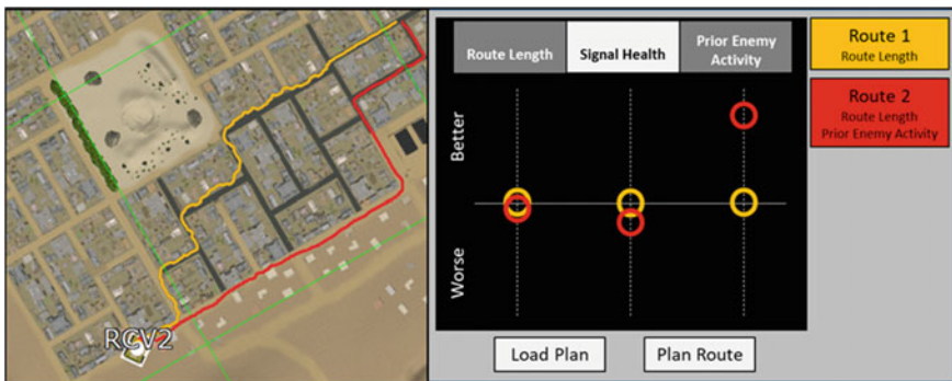
Fig. 7.5 Comparator Display prototype (right panel) along with two routes generated by the Transparent Route Planner (left panel). The Y axis of the Comparator Display is used to depict which route is better in terms of each of the mission parameters. The route shown in amber is slightly better in terms of signal health and route length. However, the route shown in red is much better in terms of avoiding prior enemy activity
