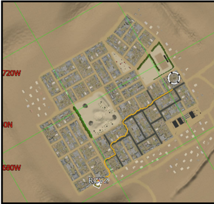
Fig. 7.4 The Transparent Route Planner has generated a route from the vehicle (labeled RCV2) to the goal location (black and white ring) using simple logic and a single click. This route plan can then be accepted or further modified by the user, increasing the team’s ability to make decisions about mobility
