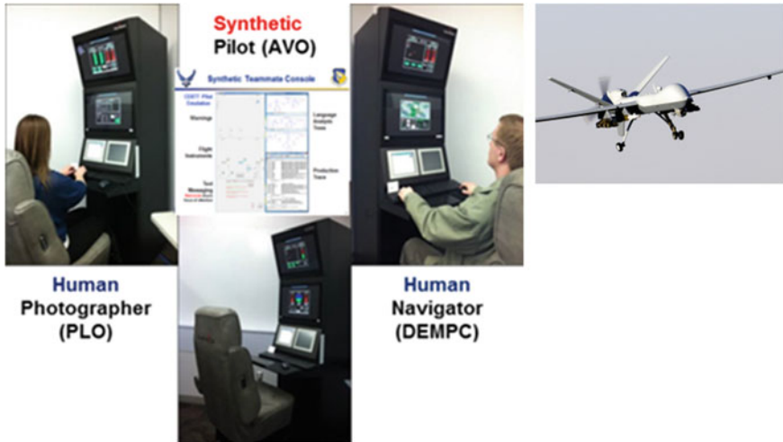
Fig. 4.5 An autonomous agent as a collaborator on a heterogeneous team (i.e., the role and nature of the agent) that operates by flying a Remotely Piloted Aircraft (RPA) to allow the team’s human photographer to take reconnaissance photos. The human photographer (PLO) and human navigator (DEMPC) have been kept in the same roles in this simulated RPAS as they held in Fig. 4.3. The air vehicle operator was an ACT-R cognitive model. By introducing the Synthetic Pilot, several implications arise regarding Interactive Team Cognition (ITC) for the Synthetic Teammate: First, the interaction goes well beyond language understanding and generation. Second, coordination among team members is central to this task; timely and adaptive passing of information among team members is affected by what the Synthetic Teammate can or cannot perform. Third, humans sometimes display subtle coordination behaviors that may be absent in or conveyed by the synthetic teammate, or even not understood by the synthetic teammate. And fourth, the failures of the synthetic teammate will highlight the requisite coordination behaviors, which we have found that a good teammate performs
