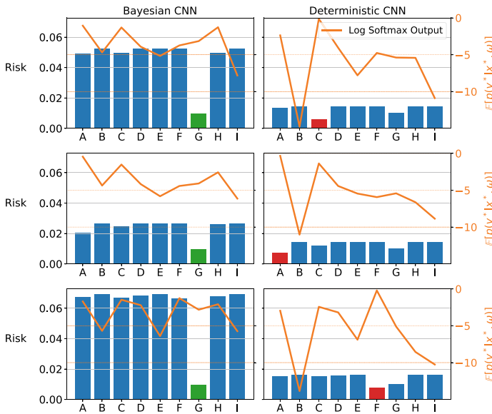
Fig. 19.4 Three example cases of how an overconfident deterministic neural network output leads to poor risk estimation and unsafe decision-making. Each row corresponds to a single audio test input for class ‘G’, and each column corresponds to the two models. For the Bayesian CNN, the lowest risk choice for all examples is the correct class ‘G’, as highlighted by the green bars. For the deterministic CNN, we see the risk is estimated incorrectly, where the risk-minimizing class decision is highlighted in red which is never class ‘G’. The overconfidence of the deterministic model can be seen from the log softmax output in orange, where the probabilities tend to fall much lower than the Bayesian CNN. This trend indicates a rather extreme confidence that such classes have almost zero probability
