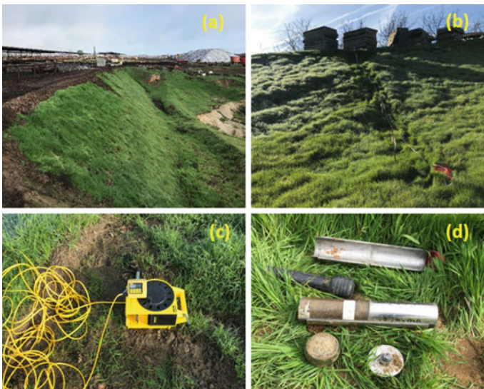
Fig. 1 Site location and details of field sampling: a grass root-reinforced slope, b slope length measurement, c altimeter, d sampling split mold
