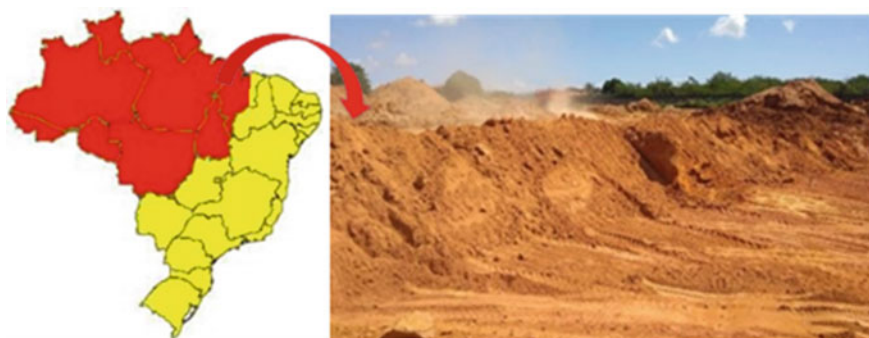
Fig. 3 Subgrade of a low traffic pavement containing a clayey sand from Sao Luis
