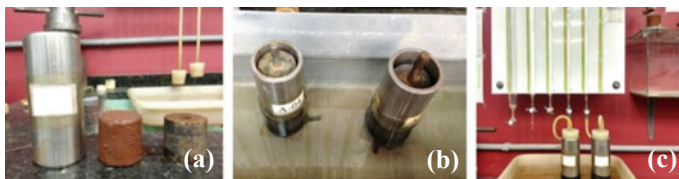
Fig. 5 VHP test for materials passing a 2.00 mm sieve: a compaction; b saturation; c test
