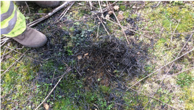
Fig. 5 Fibres present at ground surface and to a lesser degree in the exposed made ground [6]
