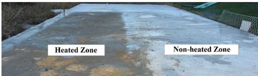
Fig. 7 Final stage of the de-icing test, the ice-free surface in the heated zone while the non-heated zone is fully covered with ice
