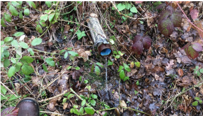
Fig. 4 Cathode at A21 stocks green. Water flowing from cathode (passive flow) [5]
