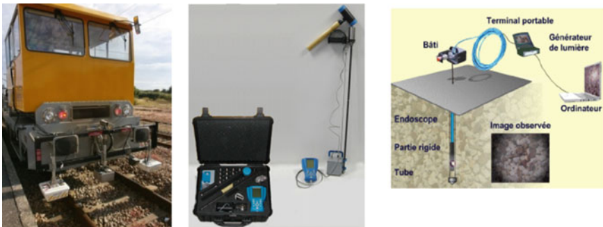
Fig. 2 Georadar vehicle (Source: Ground Control Geophysik & Consulting GmbH), PANDA ® equipment (Source: Sol Solution's PANDA ® slides and [6]) and Geoendoscopy
