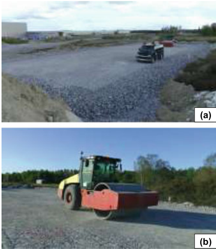
Fig. 2 Experimental setup; a trial embankment; b prototype roller; c compaction lanes
