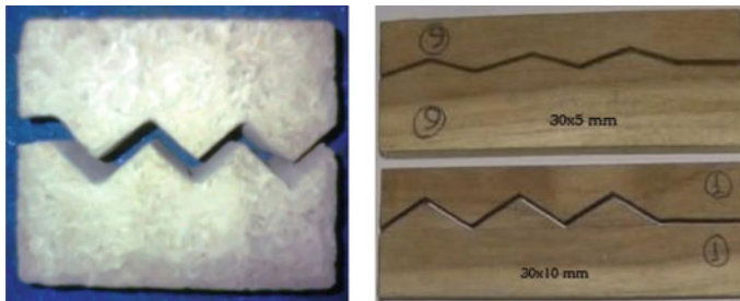
Fig. 3 Wooden blocks for asperity in cut rock specimens
