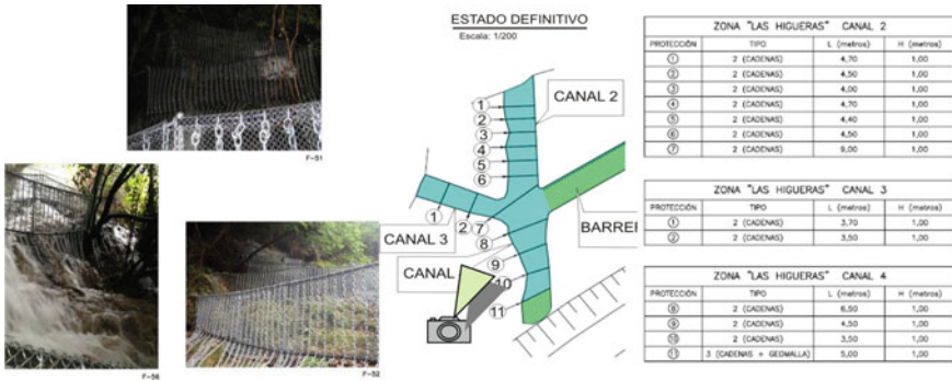
Fig. 10 Situation of the PK 169,050 MI produced by rains. Protection channels 2, 3 y 4
