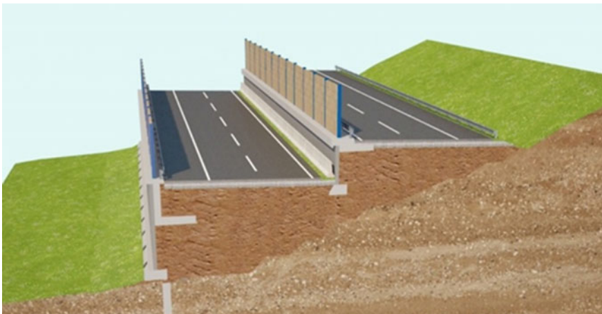
Fig. 2 Schematic cross section—highway width 24.5 m
