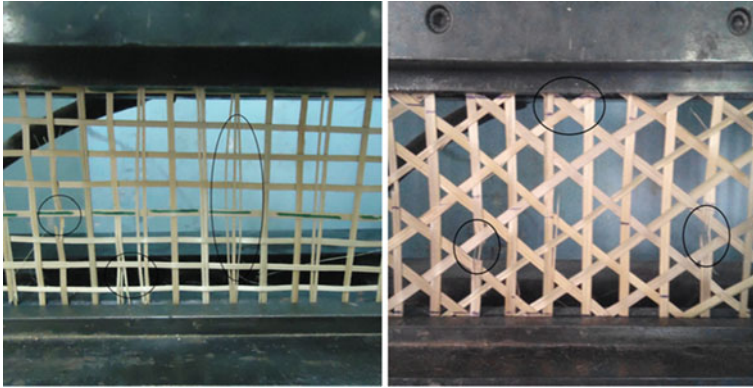
Fig. 2 Geometry of bidirectional and tridirectional bamboo grid
