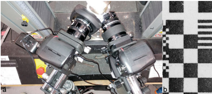
Fig. 3 a Position of cameras relative to sample in test machine and b a calibration target. Each big square is 1.429 mm across meaning that in video mode, the resolution is \sim 200 pixels per mm or 5 \mu\text{m} per pixel
