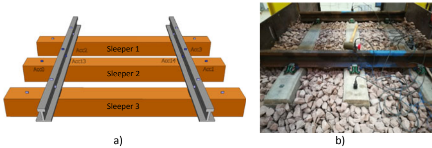
Fig. 4 Setup of the receptance test: a representation; b general perspective of the structure and setup
