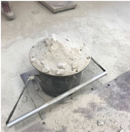
Fig. 2 Minimum density 60% fouling and 40% railroad ballast cylinder samples. On the left is the sample after being placed into the cylinder mold, and the right is after the excess is removed to the approximate correct volume
