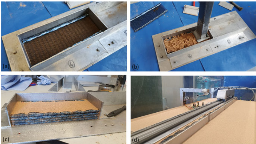
Fig. 6 a Single model geogrid and gravel bag layer in the wall former, b the fill compaction process, c a compacted 25 mm GRS-RW with four layers and d the full completed model
