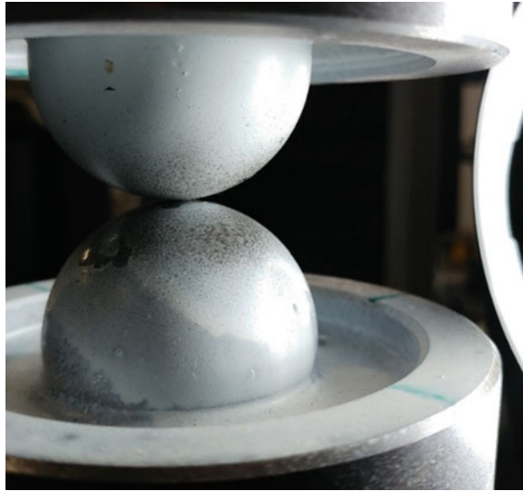
Fig. 4 Validation contact test with steel spheres of 50 mm diameter. The spheres have been sprayed white and then speckled with black spray paint to provide texture for DIC
