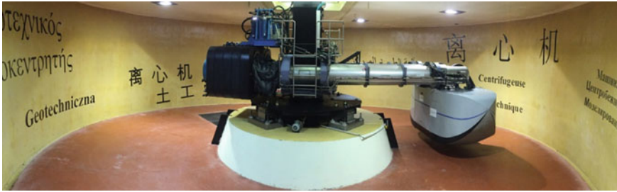
Fig. 4 Ifsttar's geotechnical centrifuge (radius 5.5 m, 2t of payload @ 100× g)
