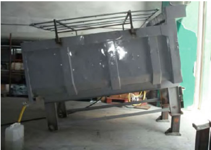
Fig. 13 Inclinable open box with a rainfall simulator
