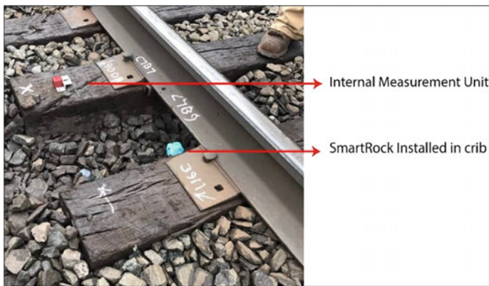
Fig. 5 Field instrumentation installation
