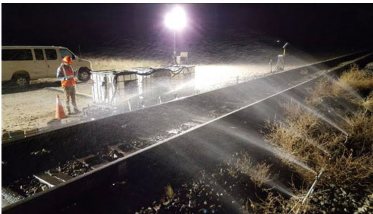
Fig. 2 Photograph of irrigation system in the rainy section
