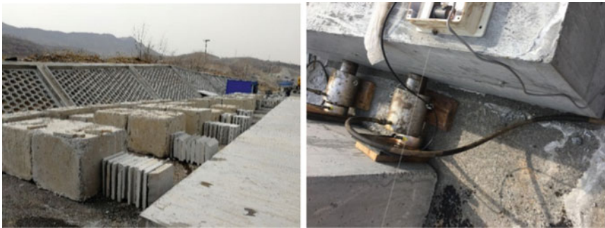
Fig. 2 Location of counter force pier and jack
