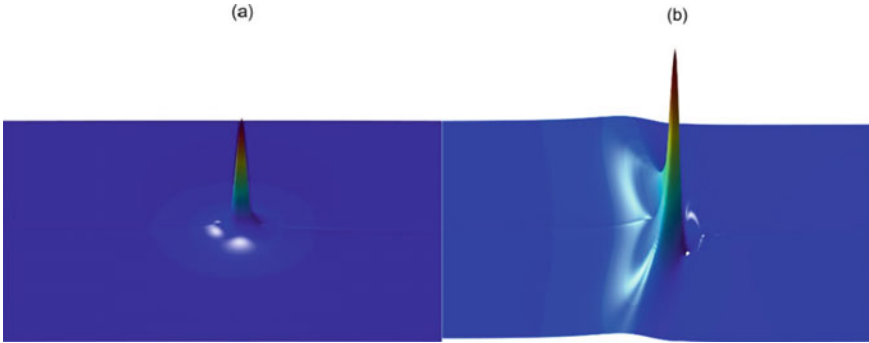
Fig. 3 Homogenous half-space soil contours: a low speed, b critical speed
