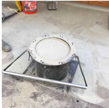
Fig. 2 Minimum density 60% fouling and 40% railroad ballast cylinder samples. On the left is the sample after being placed into the cylinder mold, and the right is after the excess is removed to the approximate correct volume
