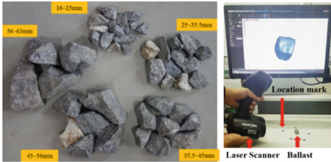
Fig. 3 Partial ballast particles used for scanning and particle scanning process
