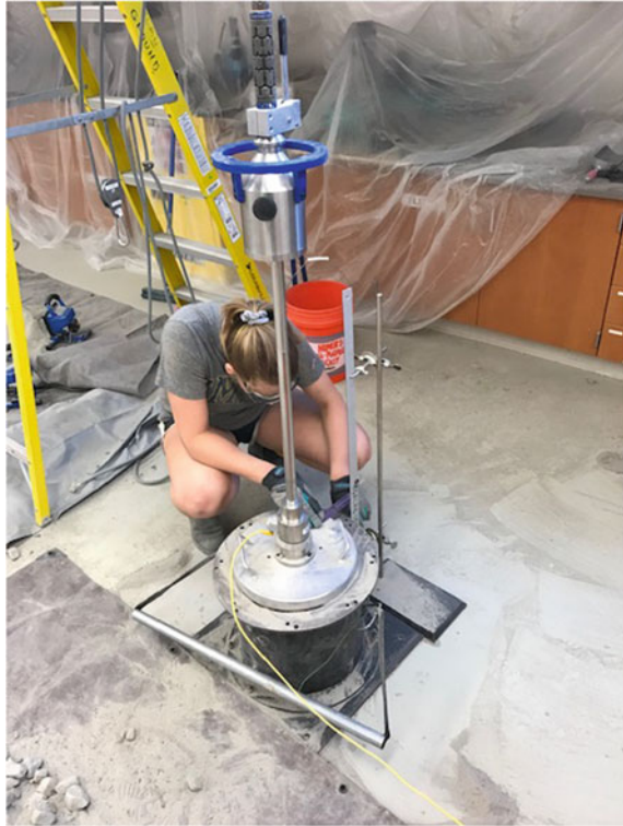
Fig. 3 Minimum density 60% fouling and 40% railroad ballast cylinder sample with LWD placed on top
