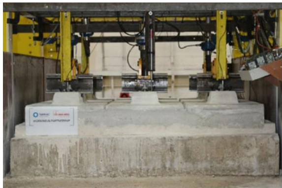
Fig. 2 Example of segments of rails (three) in a ballastless track used in the cyclic tests [15]
