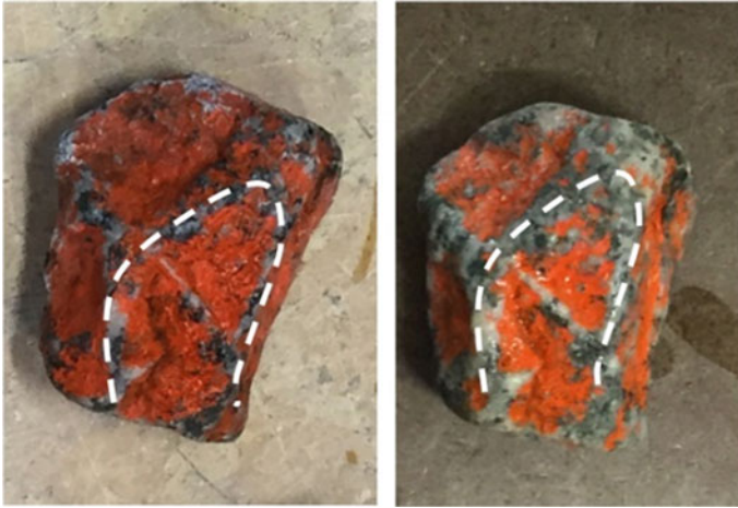
Fig. 6 Aspects of particle 1 after 2000 (left) and 14,000 (right) revolutions [24]
