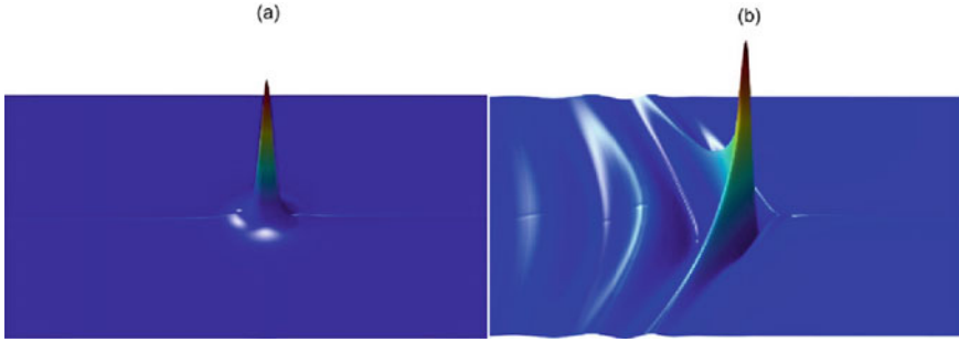
Fig. 6 Layered soil contours: a low speed, b critical speed
