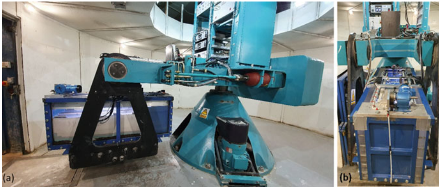
Fig. 5 a 3 m radius geotechnical centrifuge at the University of Dundee with the railway testing apparatus in place and b the model container and actuation system
