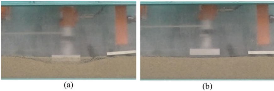
Fig. 12 State of settlement of the loaded plate after repeated loading: a D = 10 cm, L = 30 cm and b D = 2 cm, L = 120 cm
