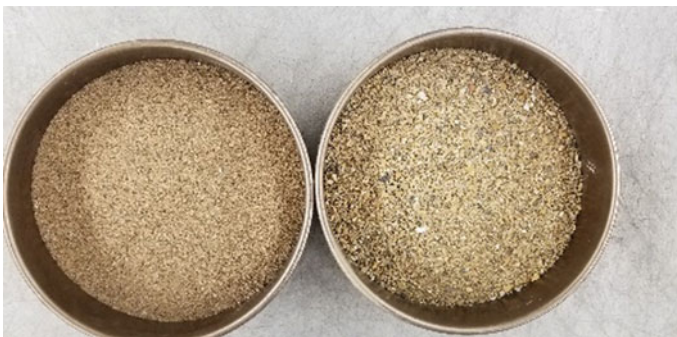
Fig. 2 Left pan shows natural sand, and right pan shows dredged material
