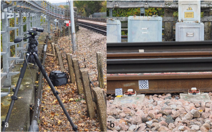
Fig. 6 Photographs of the camera setup (a) and targets on sleeper end and rail web (b)
