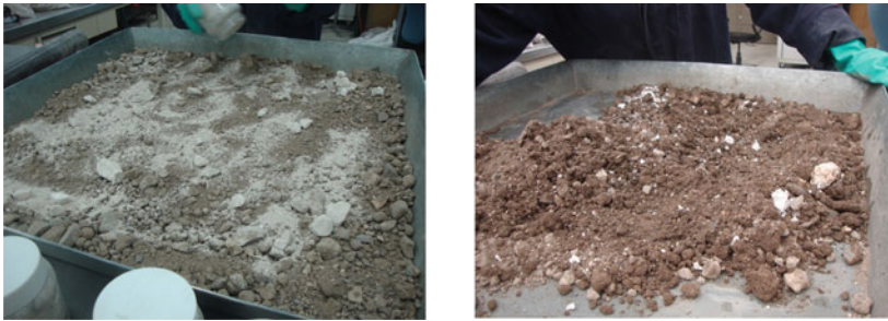
Fig. 3 Addition of calcium oxide and mixing procedure
