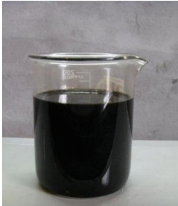
Fig. 1 Appearance of 8 wt% SMC—modified asphalt
