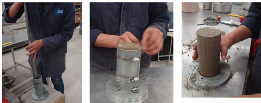
Fig. 5 Sample compaction for Guadalajara soil
