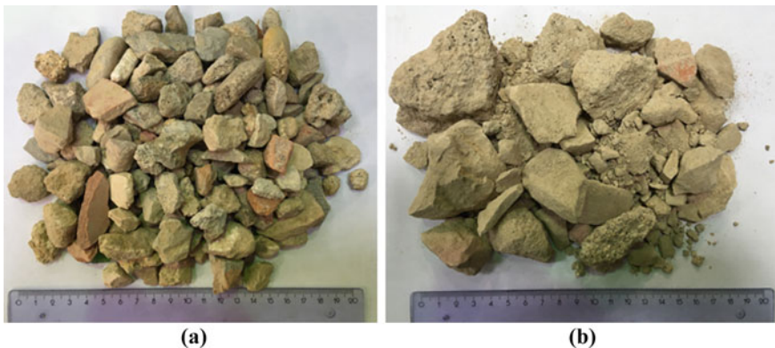
Fig. 1 Visual appearance of the recycled aggregates: a mixed C&D recycled material; b selected C&D recycled material
