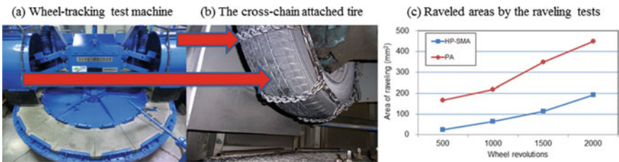
Fig. 5 Wheel-tracking test machine and raveled area as determined by raveling test
