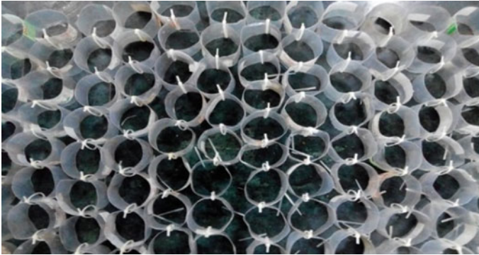
Fig. 1 Geocells cut from waste HDPE bottles
