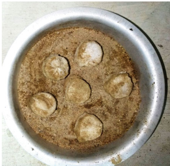
Fig. 1 Arrangement for the cyclic wetting and drying process in sand bath and wrapping of the samples with adsorptive cloth
