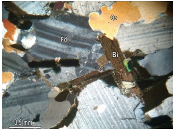
Fig. 3 Crystalline rock texture of dixcove granite: quartz, (Qz), feldspars (Fd), biotite (Bi), and fine muscovite; crossed polars
