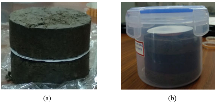
Fig. 1 Placement of filter paper for measurement of matric and total suction. a Contact filter paper for measurement of matric suction \psi_m . b Non-contact filter paper for measurement of total suction, \psi_t
