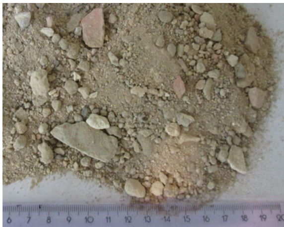
Fig. 1 Visual appearance of the C&D recycled material (ruler in cms)
