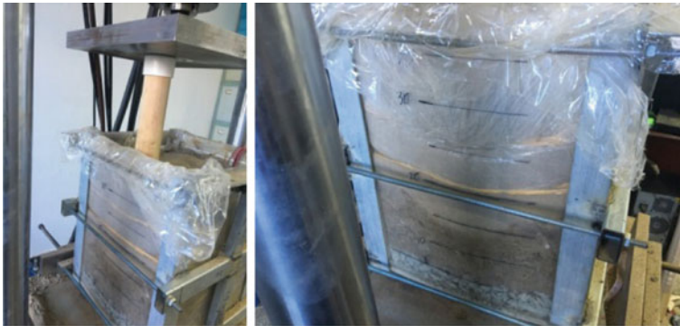
Fig. 2 Failure test of reinforced mesh cushion
