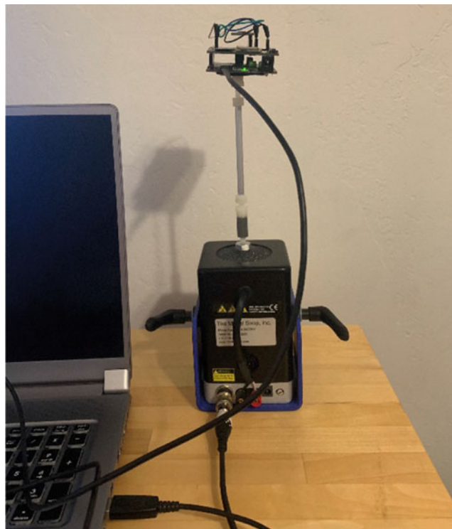
Fig. 4 Experimental setup—sensor-shaker configuration
