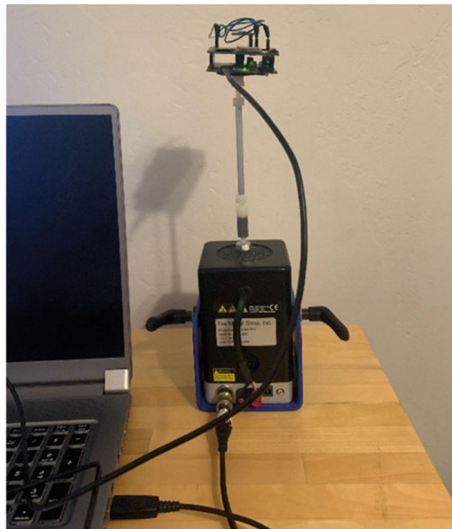
Fig. 4 Experimental setup—sensor-shaker configuration
