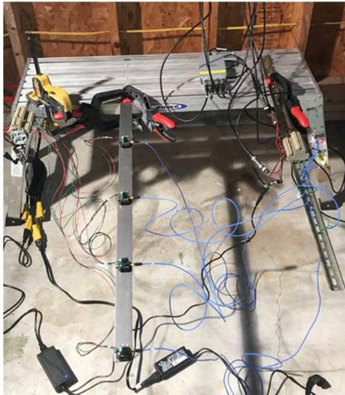
Fig. 3 Photograph of the cantilever beam test setup
