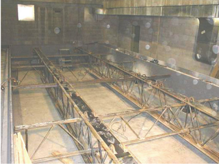
Fig. 2.8 NIST testing of steel trusses [25]
