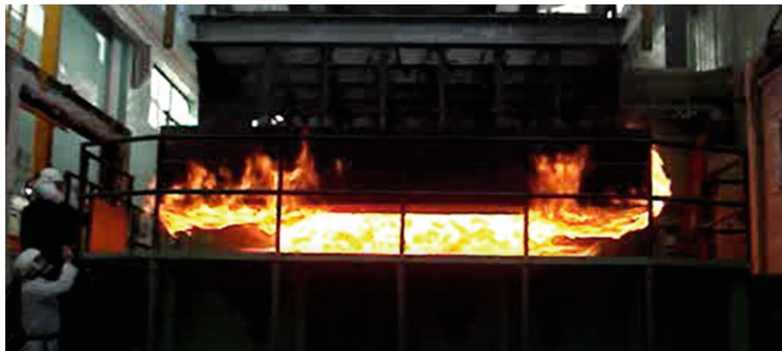
Fig. 2.5 Conclusion of a standard fire test of a wooden floor (photo by Gales)
