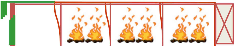
Fig. 10.3 Shear failure of a column outside the fire compartments due to thermal expansion of a floor
