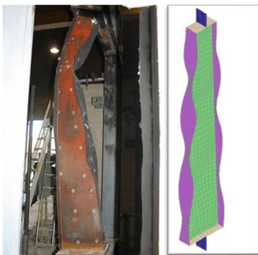
Fig. 10.6 Global failure mechanisms of a steel frame structure in fire: finite element model using beam elements in SAFIR
