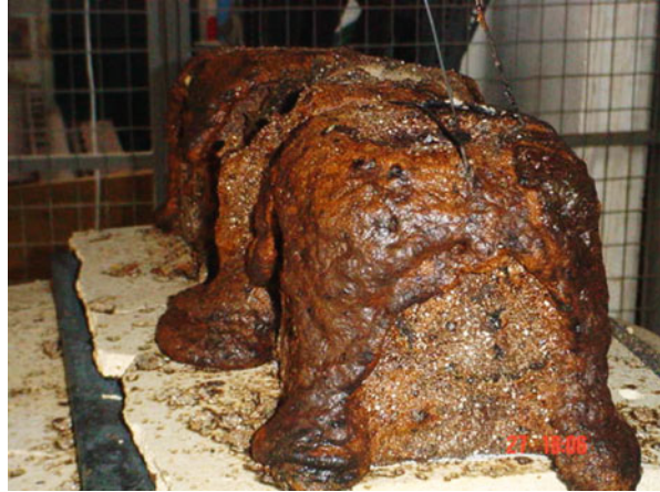
Fig. 11.26 Concrete cubes melted due to exposure to modified hydrocarbon curve (1300 °C)
