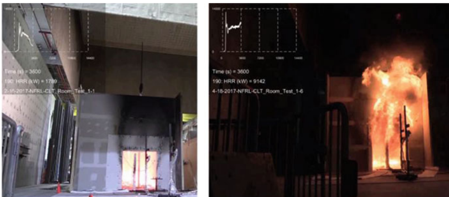
Fig. 8.24 Fully encapsulated compartment (left) and compartment with an exposed CLT wall and ceiling (right) 1 h after ignition (frame of a video by NIST, USA)
