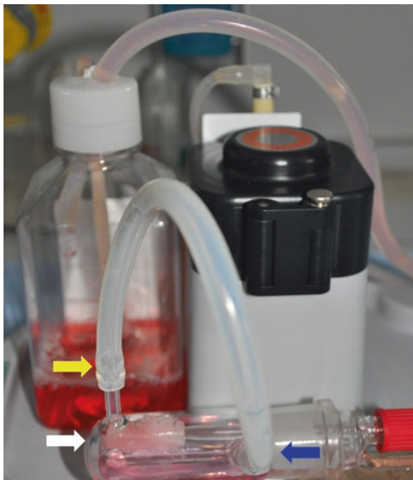
Fig. 17.2 Bioreactors specific for generation of two cell lines offering the advantages of perfusing cell-specific media on either sides of the construct due to in vitro dynamic cell culture process (white arrow: position of the cell-seeded scaffold within the bioreactor, yellow arrow and blue arrow: bioreactor access points)
