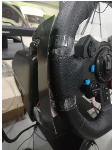
Fig. 3. The ultrasonic was created by the vibrators and transited through the horns to the display surfaces it.
