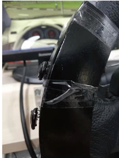
Fig. 2. The steering wheel with two solenoids embedded into each side of it.
