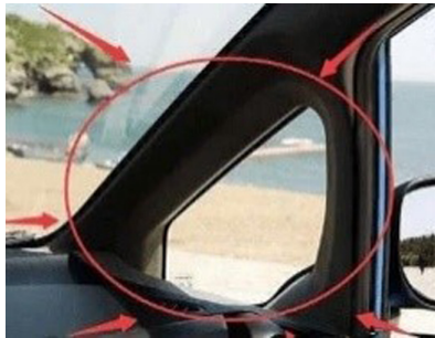
Fig. 1. Automobile manufacturer's triangular windows in front window.
