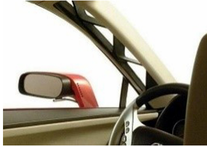
Fig. 2. Automobile A-pillar with cutout design.
