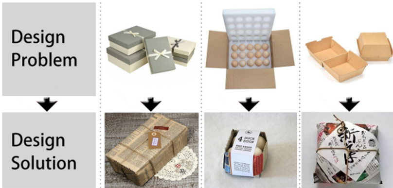
Fig. 5. The design heuristic, ‘Use waste packaging materials’, and corresponding example packagings described in the booklet
