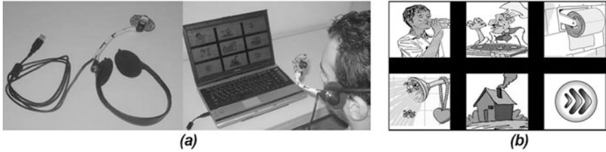
Fig. 11 A low-cost eye-tracking system for the rehabilitation of the completely locked-in patient (a) hardware set-up along with optimum position of the eyes (b) graphical user interface (GUI) representing various basic daily needs of human and the special button to ‘enable’ or ‘disable’ the buttons
