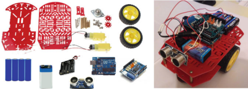
Fig. 3 Basic components of a rover (left) and the final result after assembly (right)
