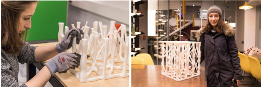
Fig. 7 A prototype printed on a 1:1 scale using FDM 3D printing technology
